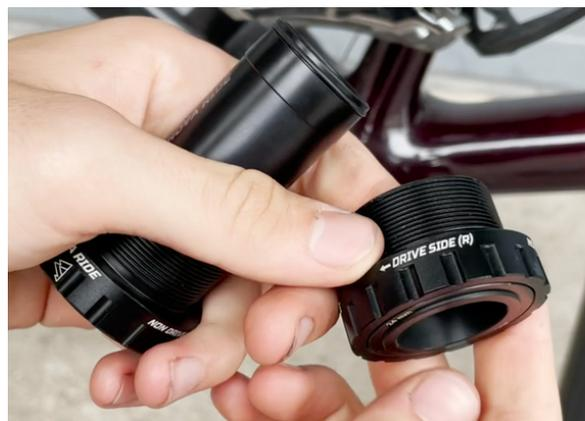
**Screw the left cup with the sealing piece into the frame on the non drive side by hand in a clockwise direction.**
